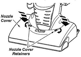
Make sure the nozzle cover retainers are in the UNLOCK position. Hook the front of the nozzle cover on to the nozzle base and rotate downward. Once in place, rotate the nozzle cover retainers to the LOCK position.
